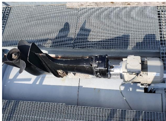
Figure 3. The propulsion system of the water tunnel [Authors' photos]
