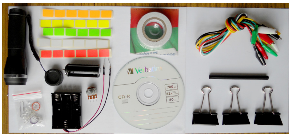
Figure 1. Details of the set-up given to the participants: 1 small plastic bag containing 8 light emitting diodes (LED), 1 paper clip and 2 small rubber rings, 1 potentiometer, 1 piece of black plastic straw, 3 metal binder clips, 1 battery holder for 3 AA-type batteries, 1 double sided adhesive tape, 1 compact disk (CD), 7 connecting crocodile cables, 1 torch with battery holder taken out, 5 bands of 6 differently colored sticky labels
