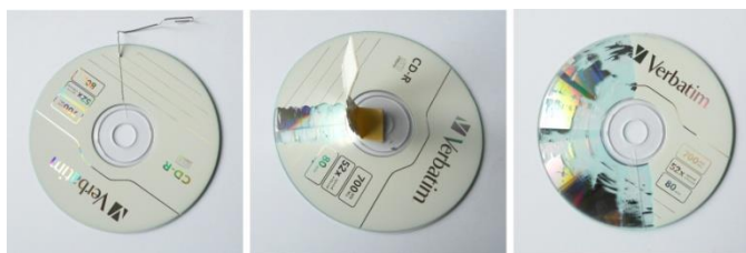
Figure 6. The technology of peeling the foil of the compact disk: 1) The foil is scratched radially with the paper clip. 2) A piece of the adhesive tape is stuck on the scratch. 3) Then the piece is pulled, and the foil stuck on the tape is removed from the CD. 4) Repeat steps 2) and 3) above (or near) the edges of the remaining foil until about half part of the disc is peeled from the foil as a half Moon at the right. You can use both sides of the double adhesive band
