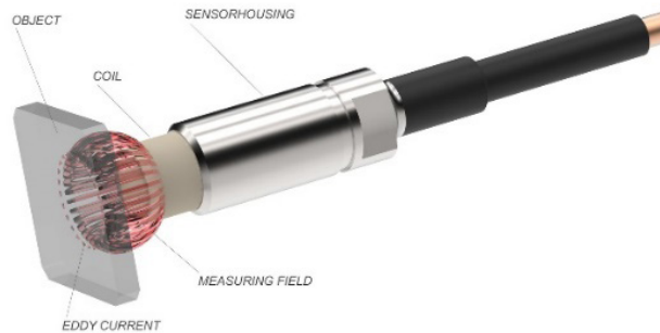
Figure 6. Eddy current sensor (eddylab 2020)
