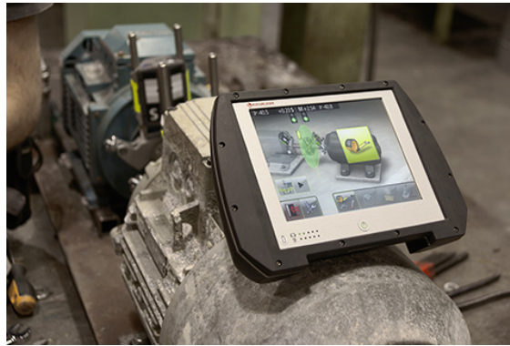
Figure 2. Laser shaft laser alignment (ACOEM Fixturelaser 2020)
