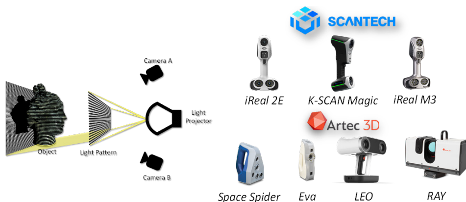
Figure 3. The principles of 3D scanning using structured light scanners (left) and a set of structured light and laser 3D scanners (right), which are used in the educational and scientific activities of the University of Ruse in Bulgaria
