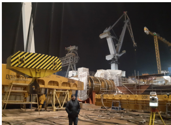
Figure 2. View of the load block and total station theodolite during measurements at the Crist S.A. shipyard
