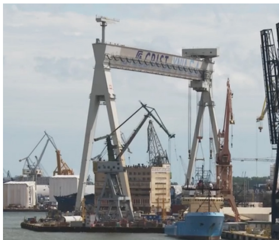
Figure 1. Gantry crane with a 1000 t lifting capacity in Crist S.A. shipyard 1)
