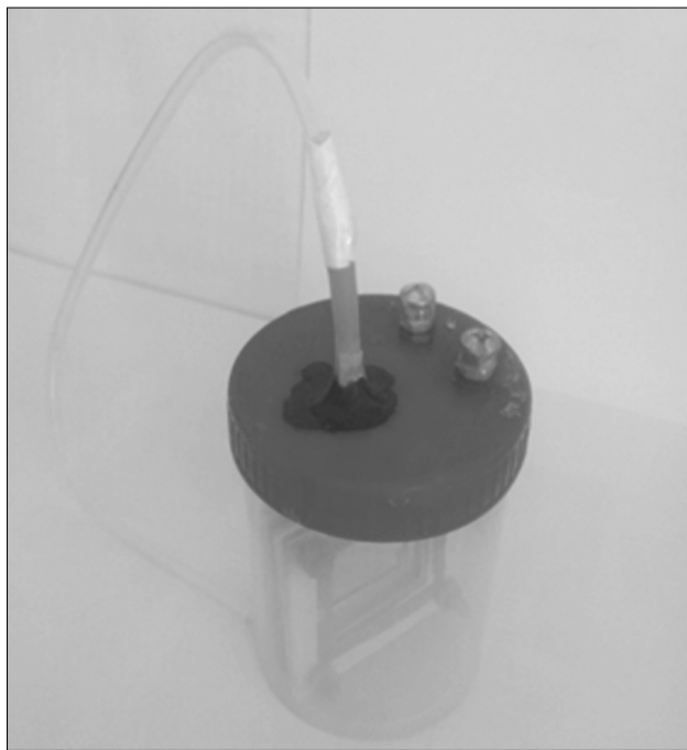
Fig. 1. Photograph of a single-chamber membrane-free MEC reactor
