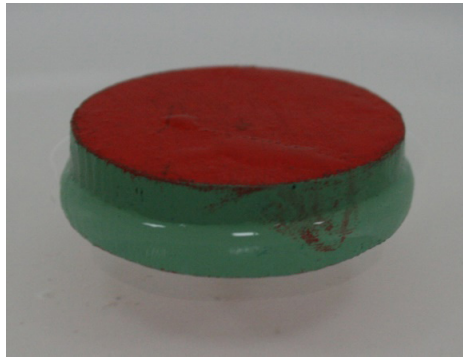
Figure 10.1. The stable floating position of the shortest cylinder
