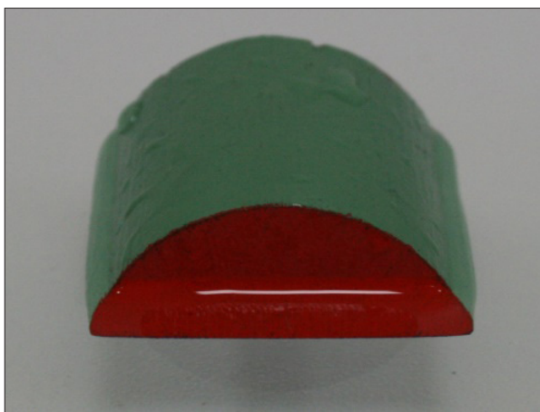
Figure 20.1. A half-cylinder in a stable floating position with the flat down
