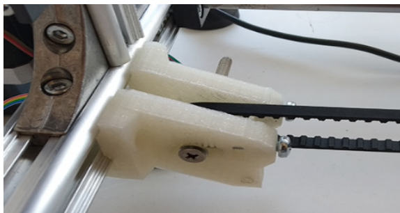
Figure 7. Mounted X-axis belt tensioner
