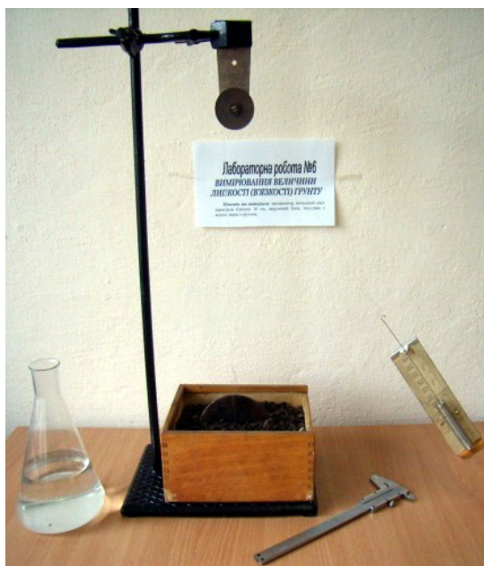
Figure 3. Determination of soil viscosity
