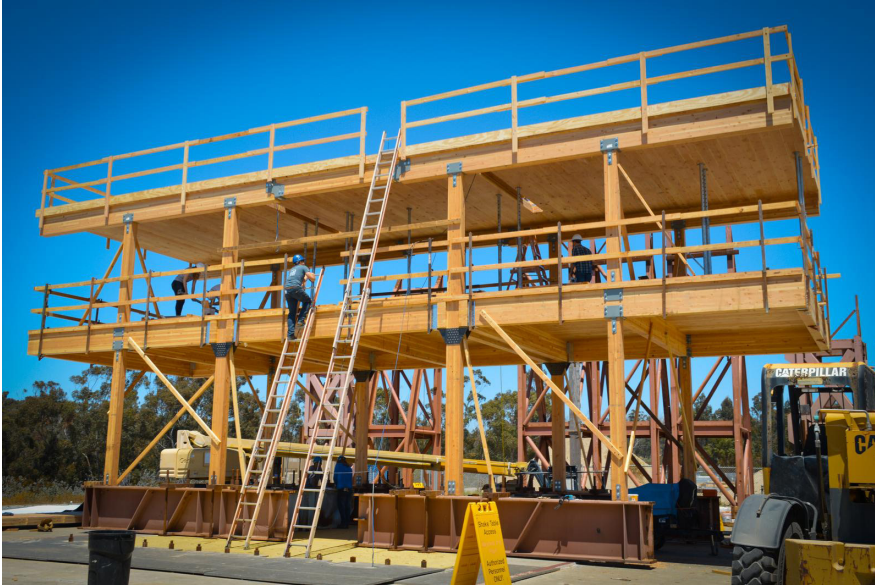
Figure 1. Earthquake shake table tests of a 20-story earthquake-resistant timber building at UC San Diego (URL-1)
