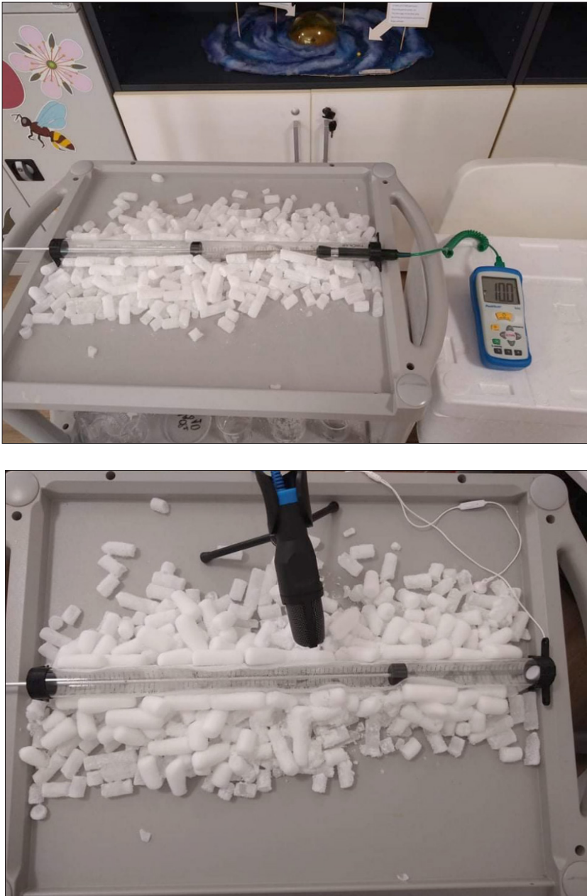
Figure 4. Dry ice used to achieve sufficiently low temperatures
