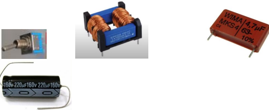
Figure 2. Switch, coil with inductivity 200 mH and condensers with capacity 4,7 µF and 220 µF.
