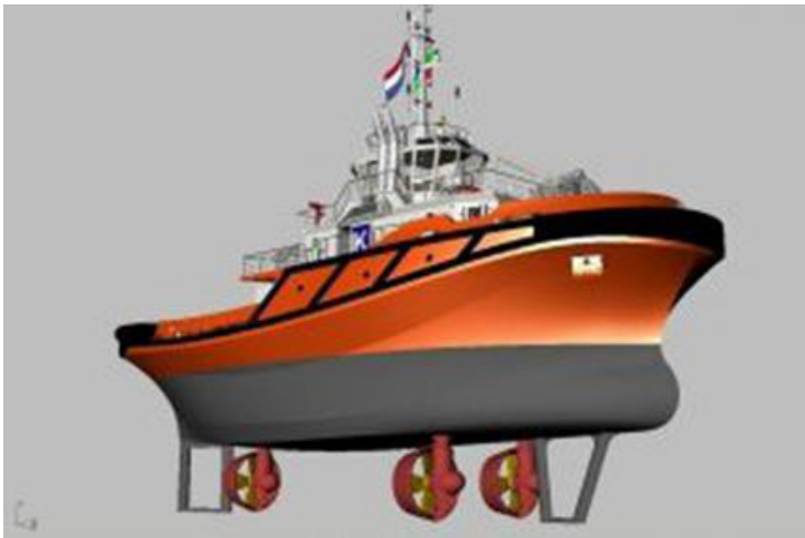
Figure 4. Rotor tug with 3 rudder-propellers 4)
