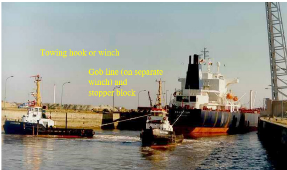
Figure 2. Conventional tug fast with stern of ship during assisting 4)
