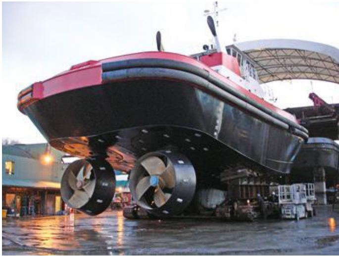
Figure 3. Azimuth thrusters on the stern 4)
