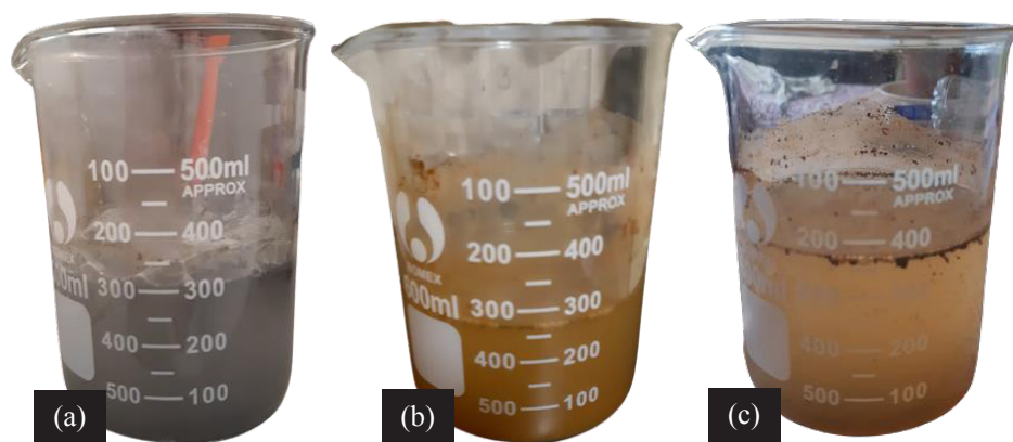
Figure 7. (a) The zinc solution before adding anything and after heating up; (b) The zinc solution after the immersion of the nickel coins; (c) The zinc solution after the immersion of aluminum foil
