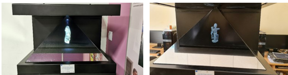
Figure 16. Hologram displays with 270-degree view angle
