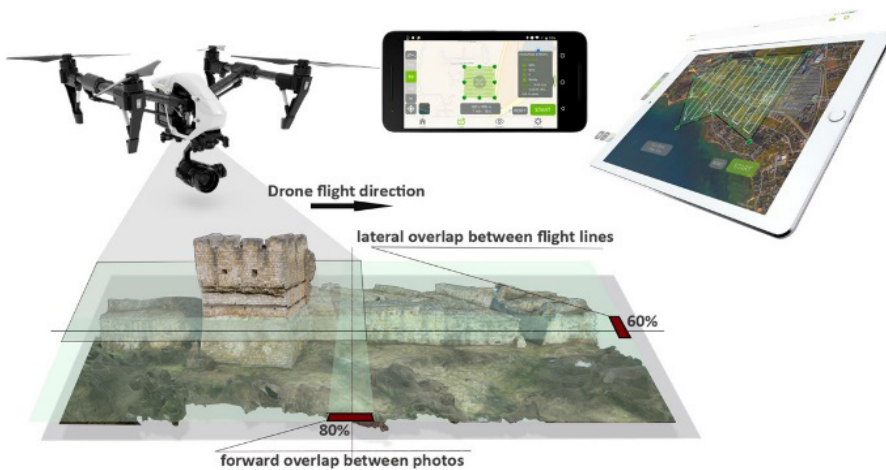
Figure 3. The principles of the photogrammetry can be used to create 3D models of buildings, geographical locations, historical sites and monuments by using drones and aerial photos
